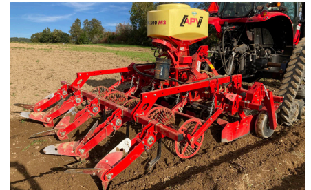
Picture 2. The APV air seeder for seeding cover crops.
