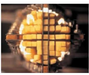
TOP: Knives are inserted into the knife box, which is similar to a cannon barrel: potatoes are fired through it. BOTTOM: Potato strips emerge from a water cutter.
