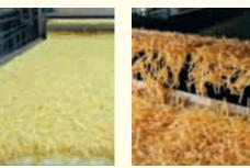
7. After drying, the potato strips are put on the equilibriation belt to balance the moisture within the potato strip.
